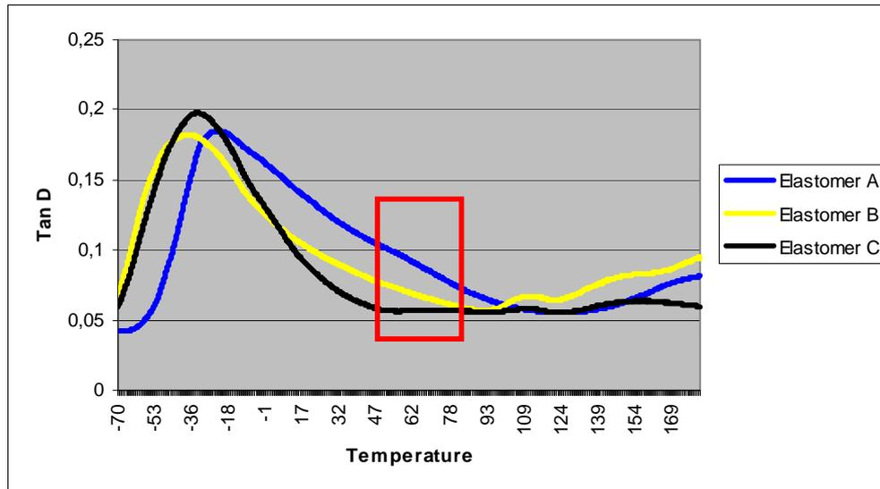
In the next stage, belts made of these elastomers were run on a shoe press of a fast newsprint machine (1750 m/min, shoe press load 950 kN/m). This machine suffered from severe wear of belts, average life of belts was only 6 weeks. The belts were grooved to certain void volume.
